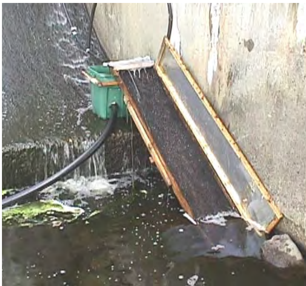
Figure 4.4.7. A “portable passage” being operated at Benton Fall Dam in Maine. The cover is lifted to show the Enkamat substrate ramp. Photo G. Wippelhauser
