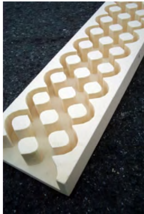
Figure 5.2. “Milieu” experimental eel pass substrate, machined from solid polyurethane foam.
